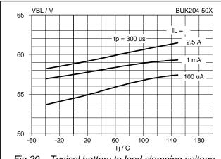
Fig.29. Typical battery to load clamping voltage.  $V_{\rm BL} = f(T_{\rm j})$ ; parameter  $I_{\rm L}$ ; condition  $I_{\rm G} = 5$  mA.
