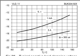
Fig.28. Typical negative load clamping voltage.  $V_{LG} = f(T_j)$ ; parameter  $I_L$ ; condition  $V_{IG} = 0$  V.
