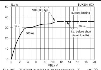
Fig.33. Typical overload characteristic,  $T_{mb}$  = 25 °C.  $I_L$  =  $f(V_{BL})$ ; condition  $V_{BG}$  = 13 V; parameter  $t_p$
