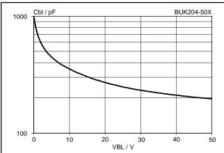
Fig.32. Typical output capacitance.  $T_{mb} = 25 \, ^{\circ}\text{C}$  $C_{bl} = f(V_{BL});$  conditions  $f = 1 \, \text{MHz}, \, V_{lG} = 0 \, \text{V}$
