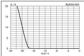
Fig.27. Typical negative load clamping characteristic.  $I_L = f(V_{LG})$ ; conditions  $V_{IG} = 0 \text{ V}$ ,  $t_p = 300 \text{ µs}$ , 25 °C
