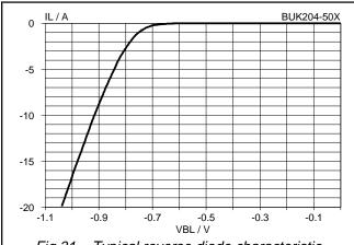
Fig.31. Typical reverse diode characteristic.  $I_L = f(V_{BL})$ ; conditions  $V_{IG} = 0$  V,  $T_i = 25$  °C
